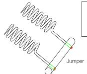
Jumper Bars to be same grade alloy as the element material. Drill holes slightly larger than wire for slip fit into jumper bar.
